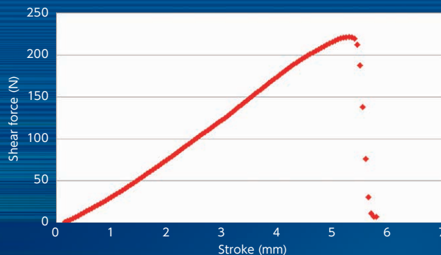
Shear force (Adherend:PET/PET)
